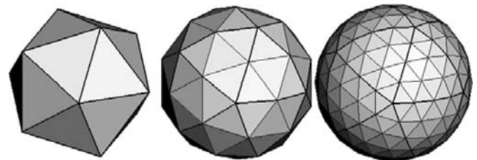
Fig. 4 Using icosahedron to generate a fine set of the wave propagation directions in 3D space
