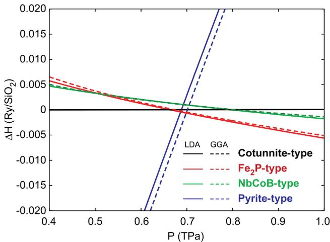
FIG. 3. (Color online) Enthalpies of pyrite-, Fe<sub>2</sub>P-, and NbCoB-type SiO<sub>2</sub> with respect to cotunnite-type SiO<sub>2</sub>.
